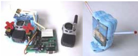
**Figure 3: Electronic prototype of the Motic Sound Display System which developed into the concept of the Programmable Puppets (PROPS)**
