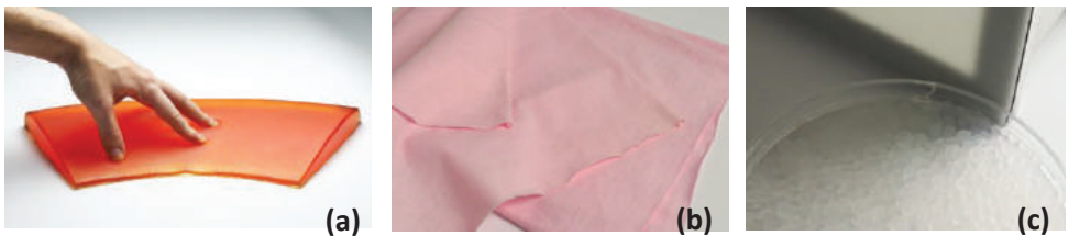
Figure 2. Experimentation with the sensorial properties of materials at Materfad, Materials Centre of Barcelona. (a) Polyurethane gel (touch properties), (b) Fabric with aroma microcapsules (smell properties) and (c) Aerogel (visual properties). Photos courtesy of Materfad.
