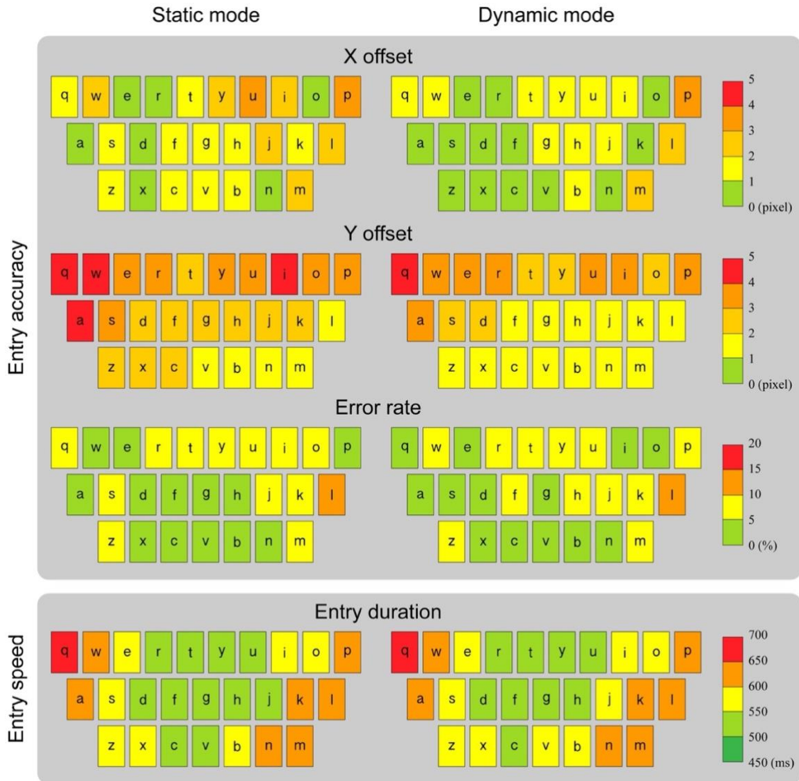
Figure 4. Heat maps for the four indices in static or dynamic modes (left column: static mode; right column: dynamic mode).
