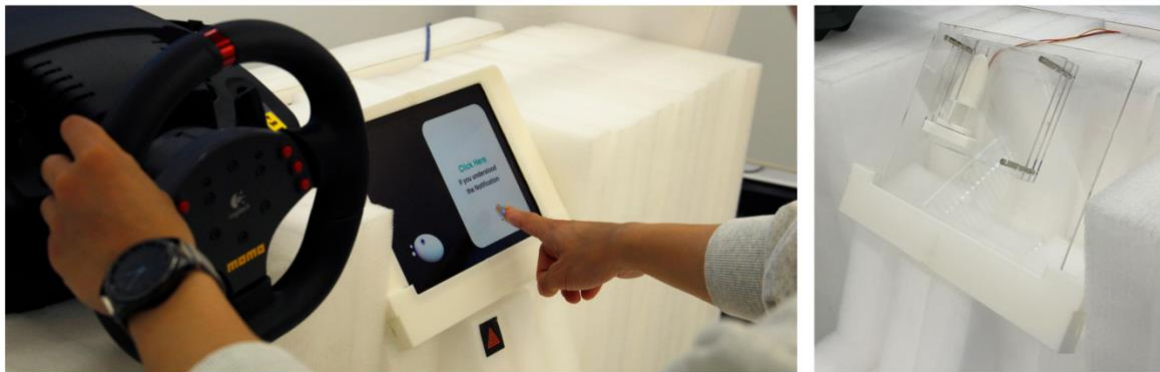
Figure 3: (Left) For measuring reaction time, the participant touching the right area on the center-fascia screen, (Right) The hardware agent emergence structure located in the back side of the iPad.
