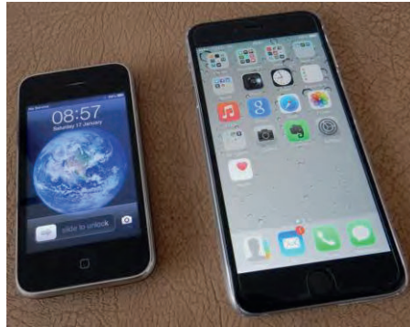
Figure 3 The 2008 iPhone 3G (left), which succeeded the original 2007 2G iPhone, was a genuine innovation with its touchscreen, icons, screen-dominated design and access to the App Store. These smartphones have been developed through five models to the 2014 iPhone 6 Plus (right) and 2015 iPhone 6s/6s Plus with larger screens and new operating systems.
