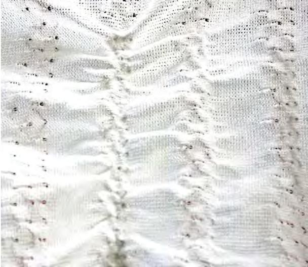
Figure 7: shaping by heat various knitted pattern in Structure 4
