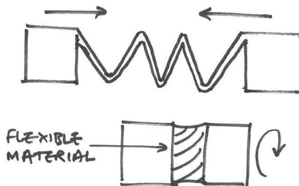
Figure 14: Compressible (a) and turning (b) structures
