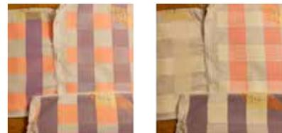
Figure 4 – the same colors in their respective cold (left) and warm (right) state.
