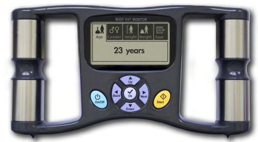
Figure 1: Virtual body fat analyser device with modified interface and controls to represent Redundant interface
