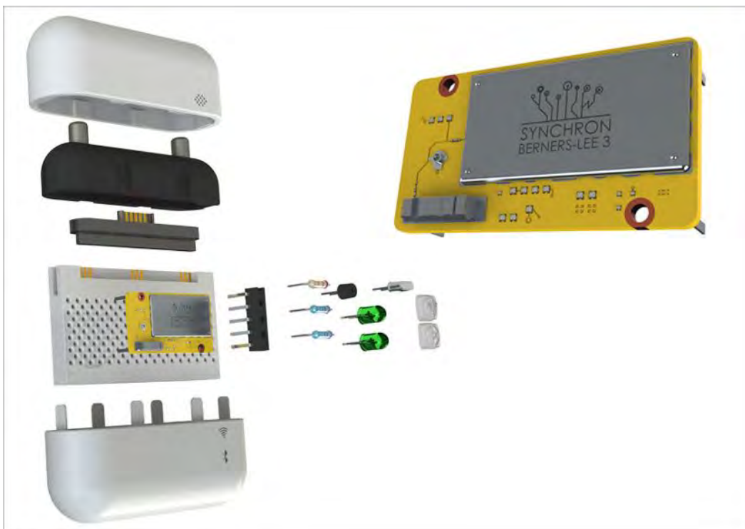
Figure 7 The design would operate via modular open source hardware and software. Here the solderless breadboard allows easy replacement/repair of componentry should any parts break. The 'Berners-Lee 3' micro-processor board's wireless and geo-locative functions enable the product and its parts to be tracked.
