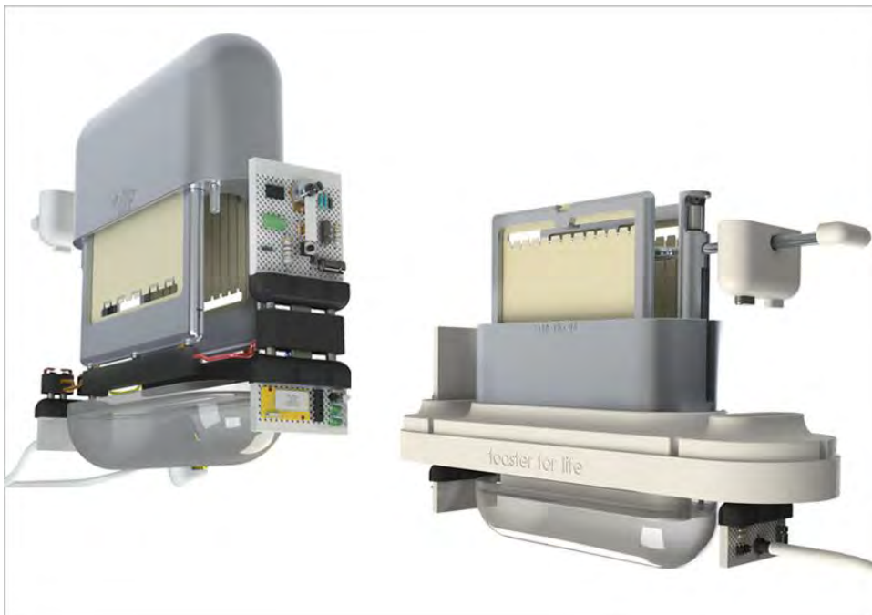
Figure 11 The Toaster For Life prototype's casing is a metaphor for 'transparency' of both form and function. It aims to entice users to open up the product and actively engage in sustainable practices including repair and upgrades. I took inspiration from these designs – Daniel Weil's 'Radio In A Bag' (left) and Freeplay's products (right).
