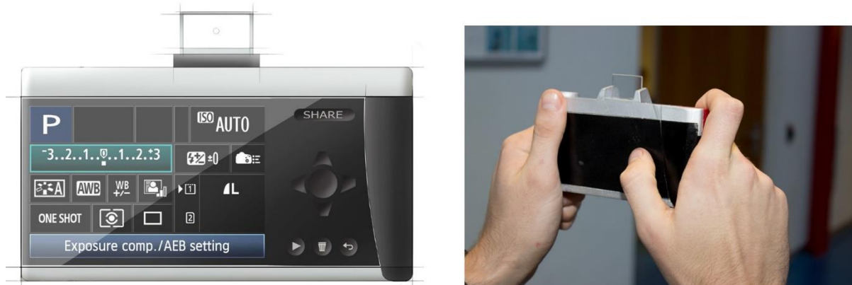
Figure 6. User interface of the future camera concept and a typical use situation holding the camera at a distance (Deinum & Feij, 2017).
