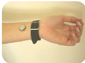
Figure 5: Thermistor placement on the internal area of the wrist of the non-dominant hand.
