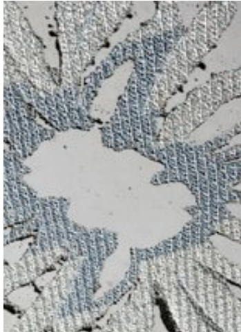
Fig2: 'stitched concrete'- textile, digitally stitched and imbedded into concrete surface gives an appearance of an embroidered surfaces
