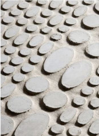
Fig1: 'linen concrete'- linen textile allows concrete mix to flow through to surface creating visual and tactile patterns
