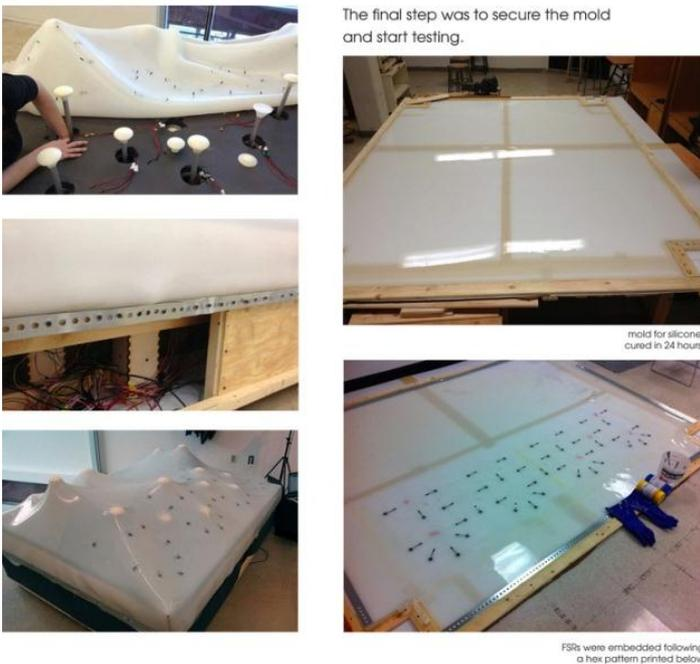
Figure 6: Custom Poured Silicone Surface Embedded With Sensors, July 2013. Photograph by Author
