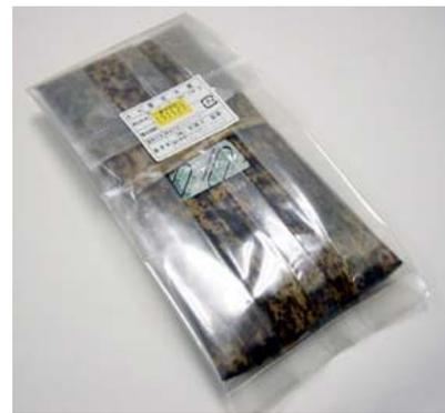
Fig. 3. Quality label, desiccant packet and plastic wrapping over the bamboo sheath
