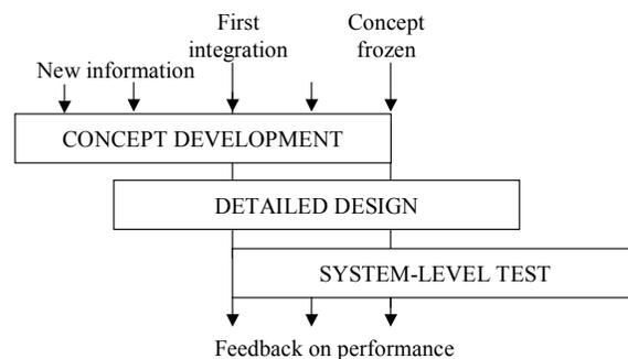
**Figure 1; flexible NPD model ( MacCormack et al 2001)**
