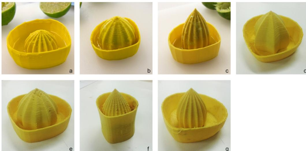
Figure 4 Prototypes (a-g) of the customized designs
