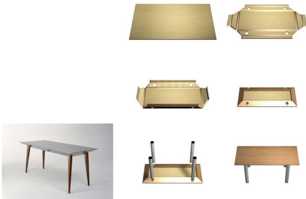
Fig. 3 Milling and folding of a table
