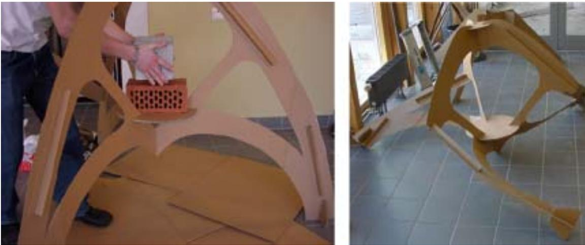
Figure 6: Loading of the structure (left) and the structure as it appeared following failure (right).
